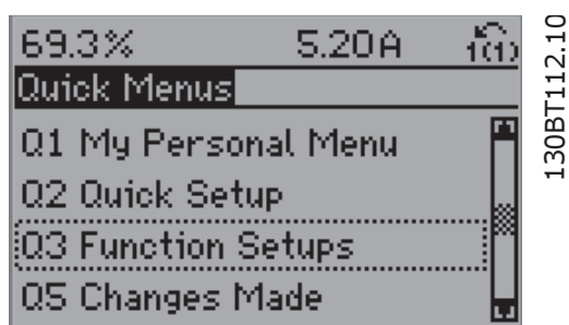
Figure 3.9: Step 3: Use the up/down navigation keys to scroll down to Function set-ups. Press [OK].
